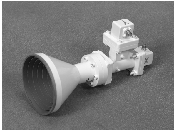
Fig. 7.4. Dual-polarized probe, made of antenna feed, for operation in the 10.7–11.7 GHz frequency range (VIC, Taiwan).
