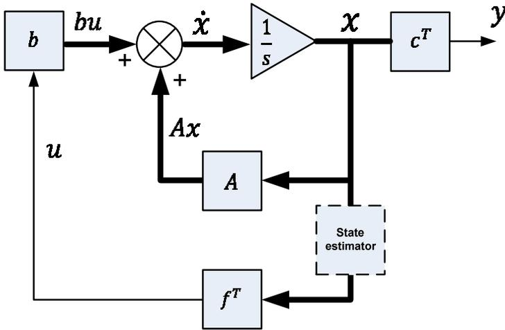
Figure 3.5 State variable feedback implementation
