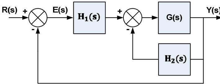
Figure 3.3 Closed loop feedforward/feedback control
