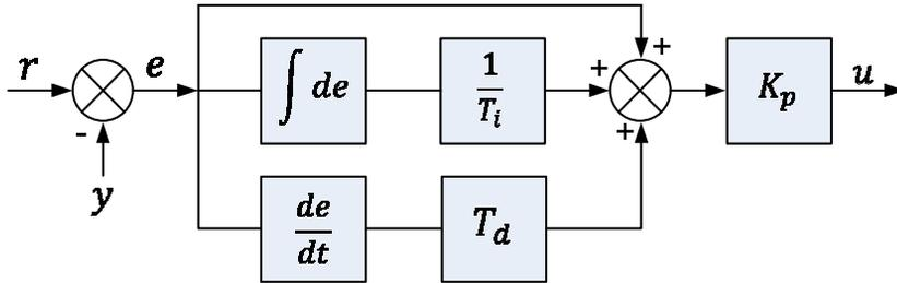
Figure 3.7 Alternative form of a PID controller
