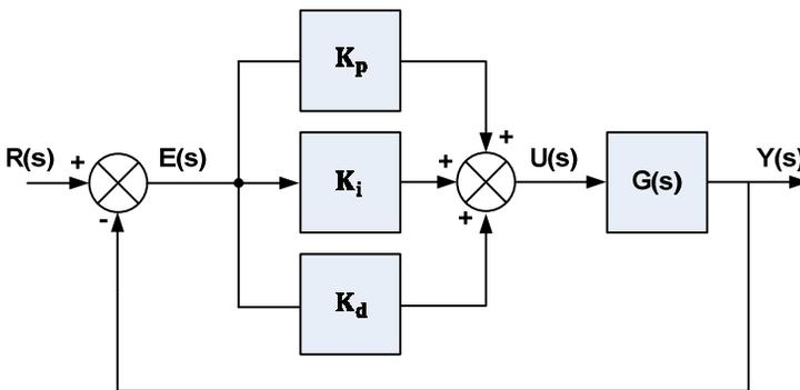
Figure 3.4 PID controller
