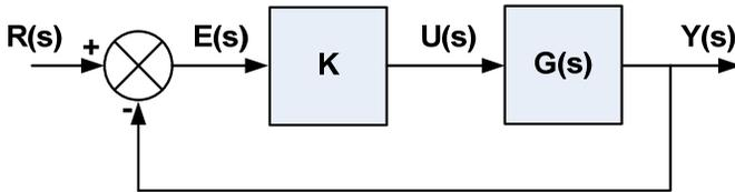
Figure 3.1 Closed-loop control
