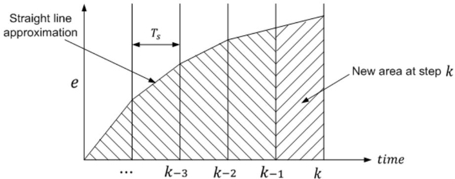
Figure 3.8 Discretisation of a continuous signal
