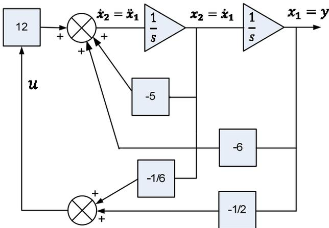
Figure 3.6 Phase variable canonical form of closed-loop system
