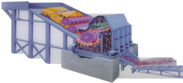
Fig 56. Scheme of a shredding installation
