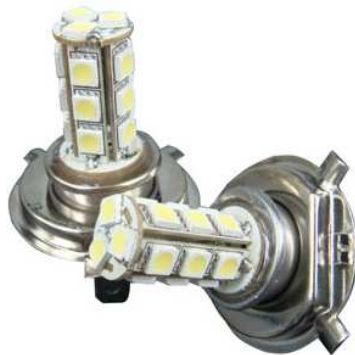
Fig. 11.16. LED car bulb [4]
