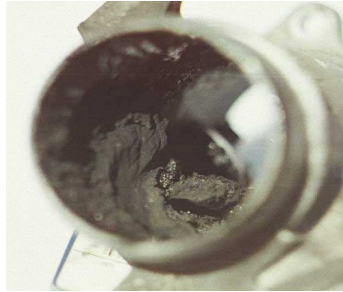
Fig. 3.13. Gummed up intake valve of EGR
