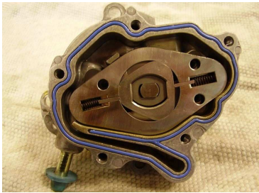
Fig.3.10. Negative-pressure pump (fuel pump is on other side)
