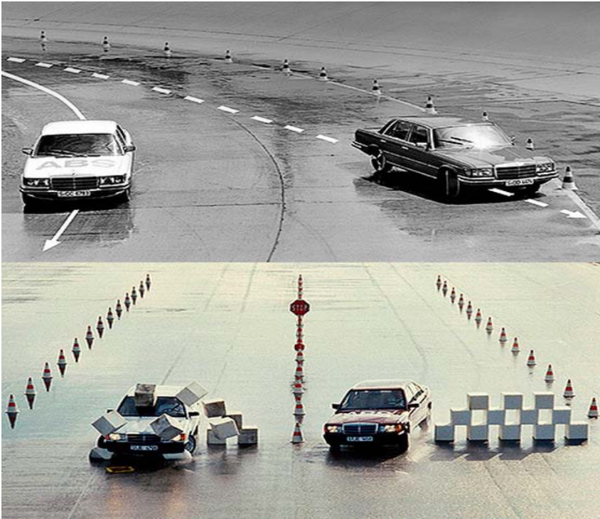
Figure 4.11 Comparison of car steerability with and without ABS
