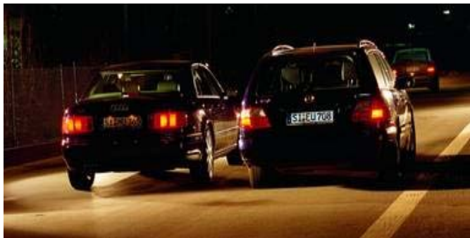
Figure 9.12 Difference in license plate visibility - from left side: standard, polycarbonate coated
