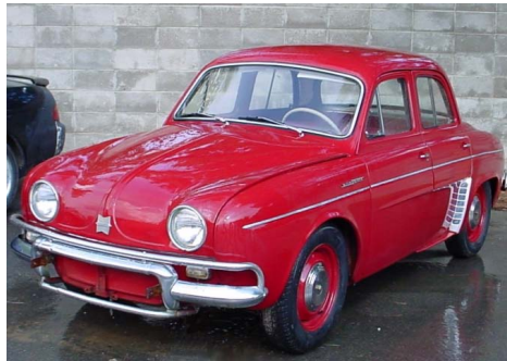
Figure 11.3 The Henney Kilowatt, the first modern (transistor-controlled) electric car. Based on a Renault Dauphine
