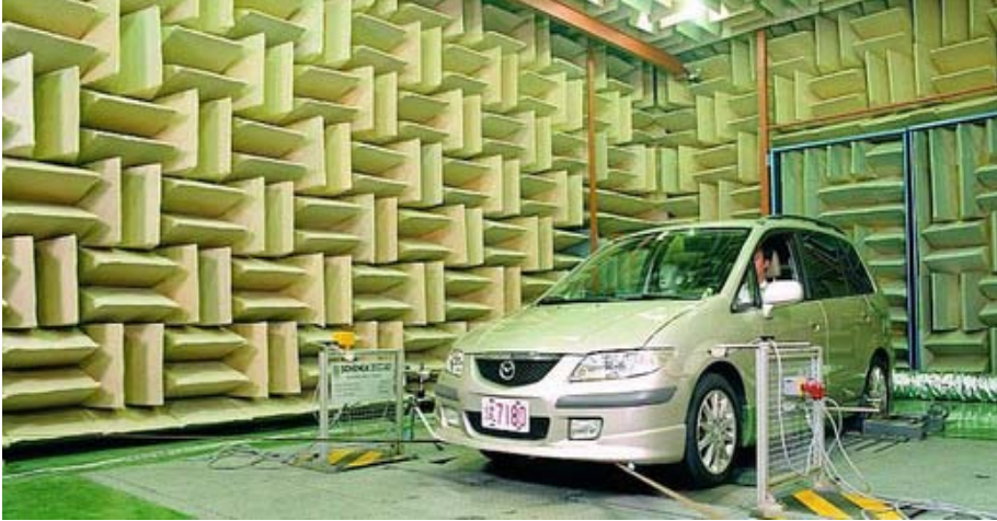
Figure 8.6 Semi anechoic chamber for noise measurements
