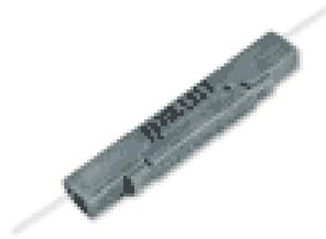
**Fig. 7.40 3M Fibrlok.**  $il < 0.2\text{dB}$ ,  $fr > 7.75\text{ lbs.}$   $orl - 35\text{dB}$ . V-groove technology - no epoxy. Thermal stability of  $-400^\circ\text{C}$  to  $800^\circ\text{C}$   $il -$  insertion loss,  $fr -$  fiber retention,  $orl -$  optical return loss.
