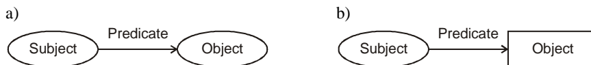
Figure 8.1. Graphical representation of an RDF triple a) subject and object nodes are resources, b) object is literal.
