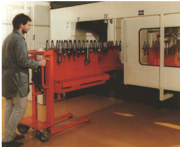
Fig. 6.25. Manual tool cassette exchanging in a tool store with stationary tools position
