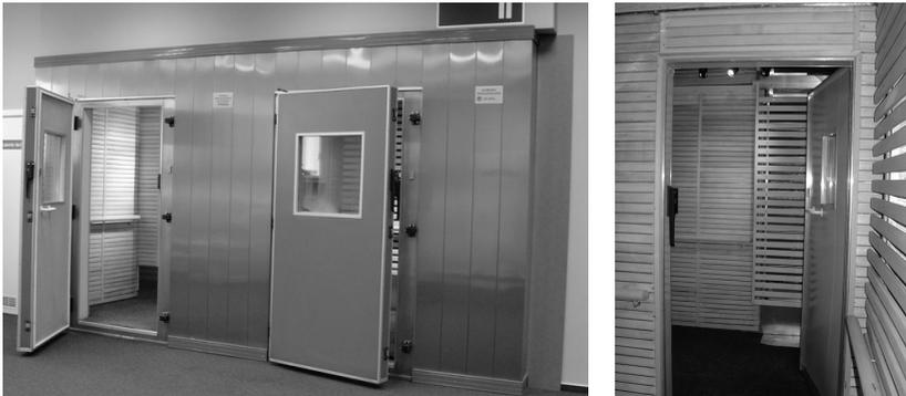
Figure 1. Cryochamber room-type
