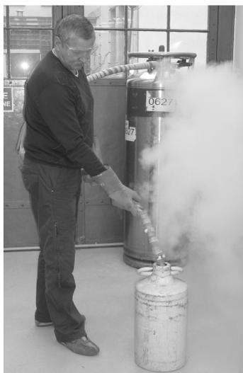
Figure 1. The technician fills Dewar with liquid nitrogen
