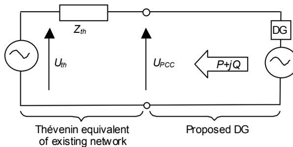
Figure 8.2 Equivalent circuit for estimating voltage rise
