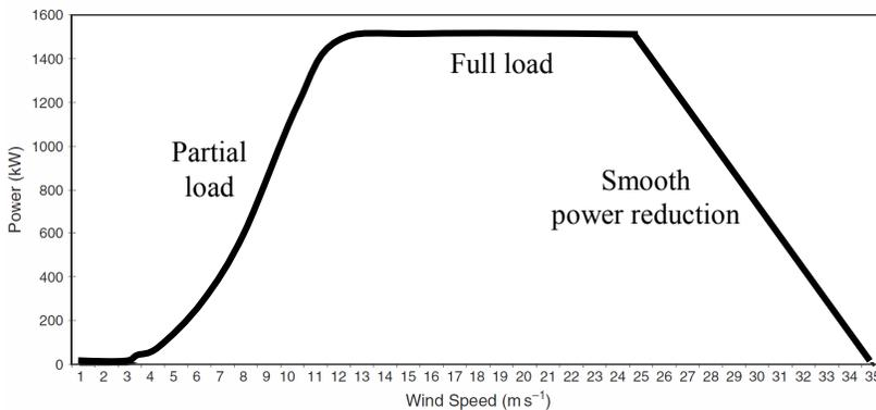
Figure 2.5 The power curve of a 1500kW pitch-regulated wind turbine with smooth power reduction during very high wind speeds
