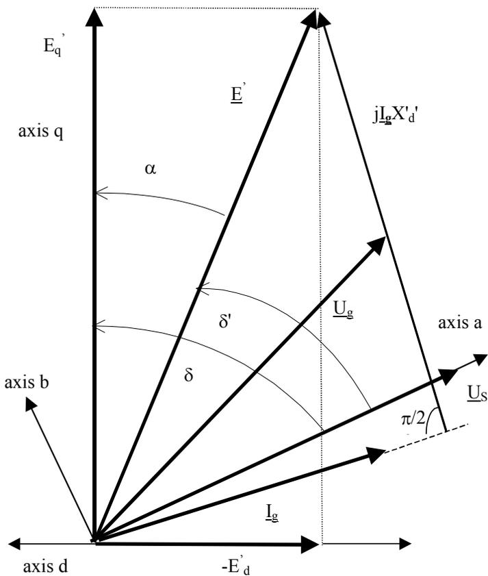
Figure 5.2. Phasor diagram of a generator in classical modeling.
