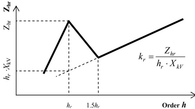
Figure 4.3 System harmonic impedance approximation, using the envelope impedance curve (IEC 61000-3-6)
