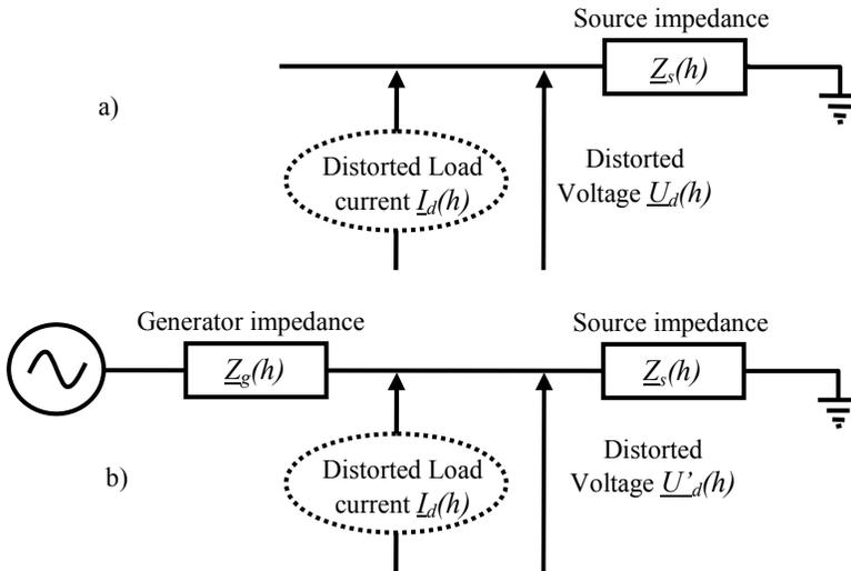
Figure 12.2 Effect of a ‘perfect’ embedded generator on network power quality
