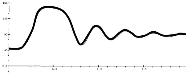
Figure 10.5 Oscillations in the rotor angle of the embedded generator at bus E following a fault at bus D when this generator produces 11.5 MW. The fault is applied at  $t = 100$  ms and cleared at  $t = 300$  ms
