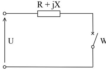
Figure 7.2. One phase representation of a 3-phase short circuit, where  $W$  depicts circuit breaker.
