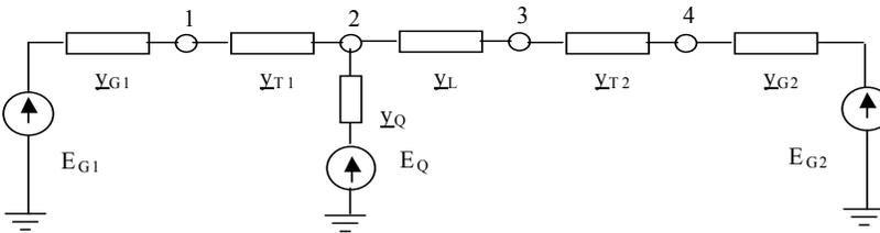
Figure 7.7 A four-bus example system (a) and its equivalent circuit (b).
