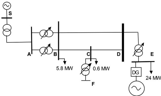
Figure 10.2 Small system used to illustrate the stability studies
