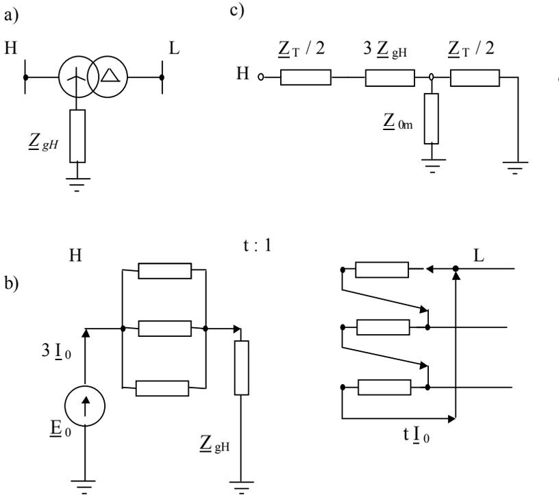
Figure 7.12 Case of YNd transformer windings, a) key diagram, b) measurement diagram, c) equivalent diagram.
