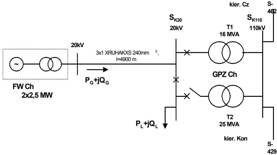
Figure 15.9 Test system for investigating the voltage control capabilities of 2 wind turbines
