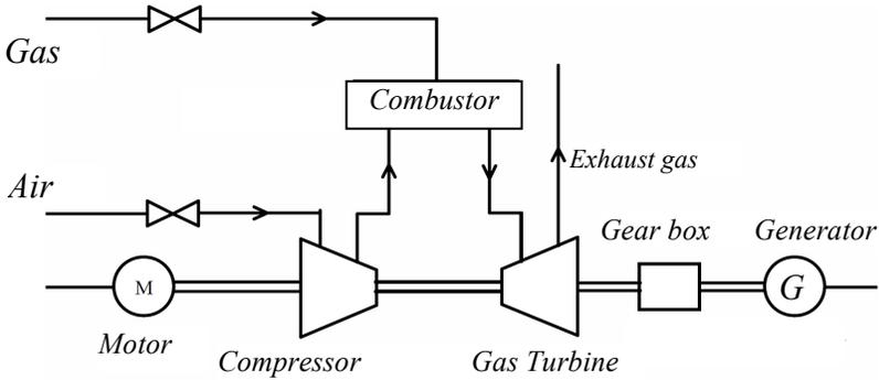
Figure 13.2 Single shaft open cycle gas turbine
