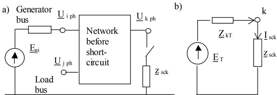
Figure 7.5. Thevenin's theorem in short-circuit analysis; a) before short-circuit, b) short-circuit with Thevenin's impedance
