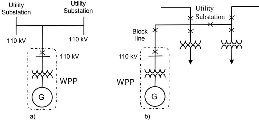
Figure 3.8 Methods for connecting Wind Power Plants to the National Power System:
