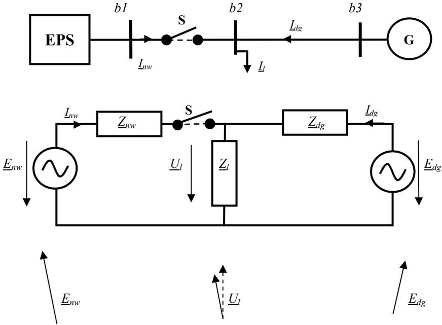
Figure 11.5 Voltage vector shift after islanding. Thevenin equivalent of the network with  $E_{nw}$ ,  $Z_{nw}$  and of the generator with  $E_{dg}$ ,  $Z_{dg}$  respectively
