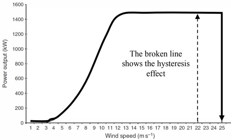
Figure 2.4 Power curve for a 1500 kW pitch regulated wind turbine with cut-out speed of  $25 \text{ m s}^{-1}$ .
