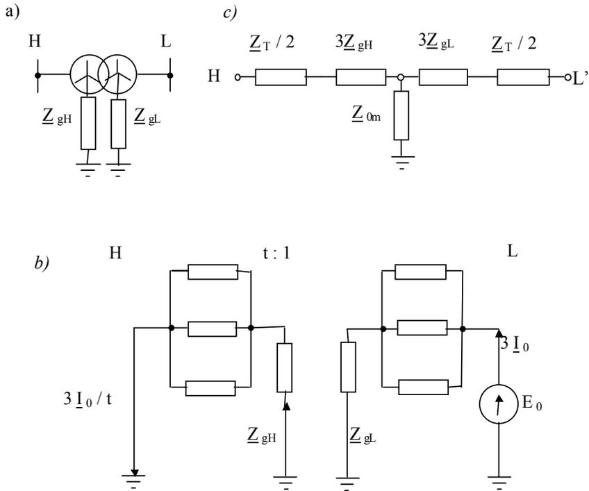
Figure 7.11 Case of YNyn transformer windings, a) key diagram, b) measurement diagram, c) equivalent diagram.
