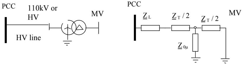
Figure 15.3 Zero sequence impedance equivalent circuit of WPS-EPS circuit.
