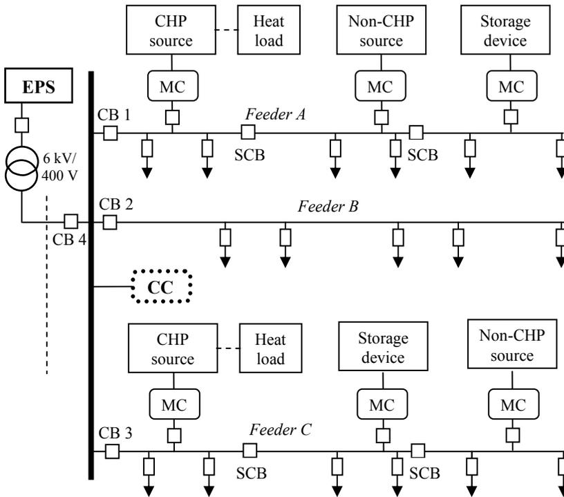
Figure 14.1 A typical Microgrid configuration: CHP – Combined heat and power, MC – Microsource controller, SCB – Sectionalizing circuit breaker, CC - Central controller, CB – Circuit breaker
