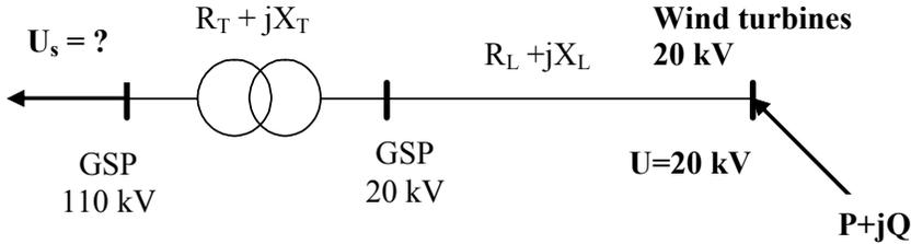
Figure 15.6 Small power system used to illustrate the WPS impact on MV distribution network
