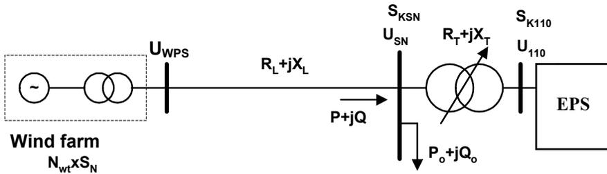
Figure 15.4 A simplified single-line diagram of the local 20 kV network with WPS used to illustrate the voltage imbalances. Note:  $N_{WT}$  - number of wind turbines are aggregated,  $S_N$  - Rated apparent power of a wind turbine,  $S_{K110}$ ,  $S_{KSN}$  - the short circuit power in the 110 kV and MV substation, respectively.
