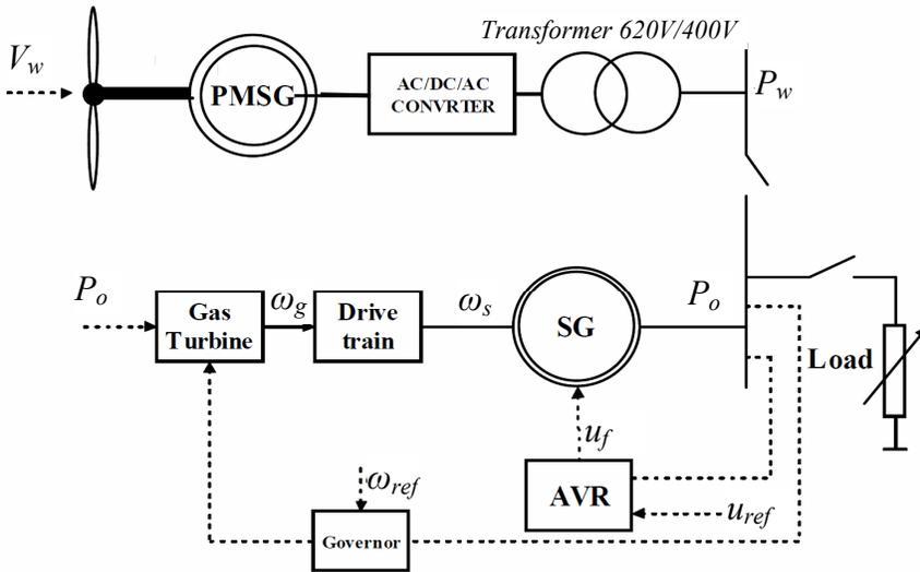
Figure 13.1 Wind-gas hybrid power system
