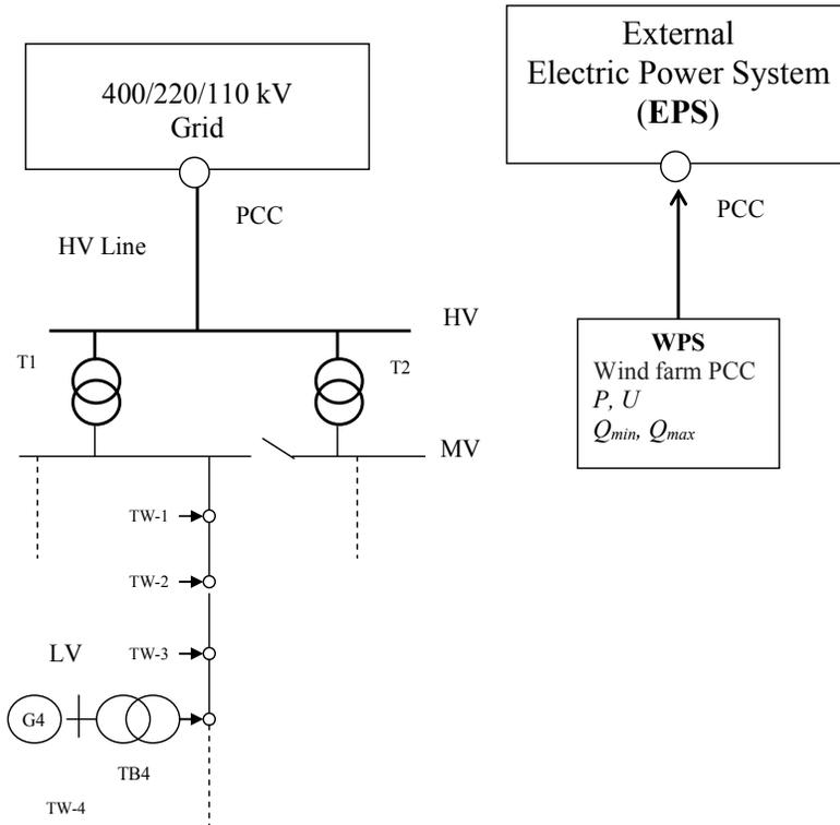
Figure 15.1 Example network with a wind farm (single line diagram and a simplified equivalent). Note: PCC - Point of Common Coupling,  $P$  – output active power from wind power,  $U$  regulated voltage at the point of PCC of the reactive power from  $Q_{min}$  to  $Q_{max}$
