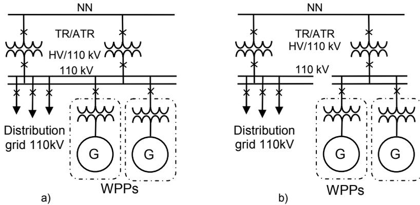
Figure 3.10 Methods for connecting Wind Power Plants to the National Power System:
