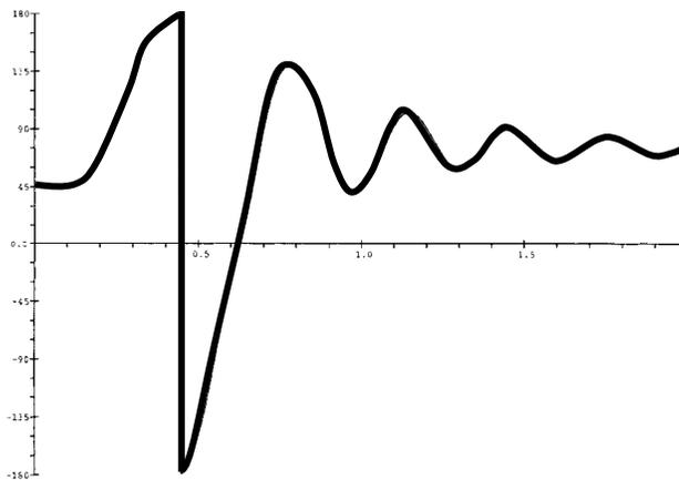
Figure 10.4 Oscillations in the rotor angle of the embedded generator at bus E following a fault at bus D when this generator produces 11.6 MW. The fault is applied at  $t = 100$  ms and cleared at  $t = 300$  ms. Note that this particular computer program keeps all angles as being between +180 degrees and -180 degrees. There is thus no discontinuity in angle at  $t = 445$  ms – simply a modulus operation
