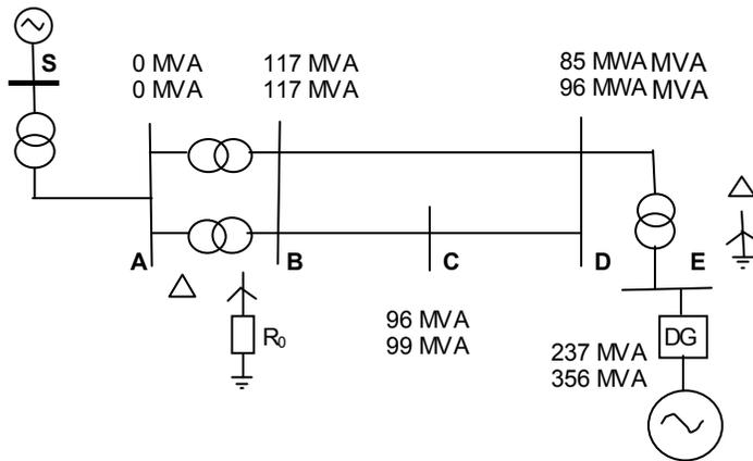
Figure 7.15 MVA fault levels for single line-to-ground faults at various buses in the system. The upper number corresponds to the case where the embedded generator is not connected to the system and the lower number to the case where it is. The system is assumed to be unloaded prior to the fault
