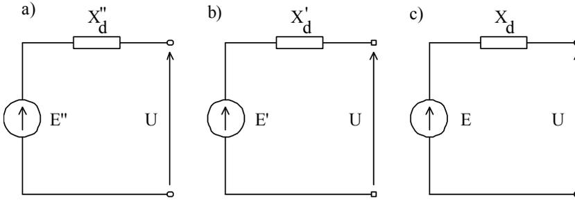
Figure 7.4. Equivalent circuits of generator in subtransient, transient and synchronous states for: (a) the subtransient period, (b) the transient period, (c) the steady-state period.
