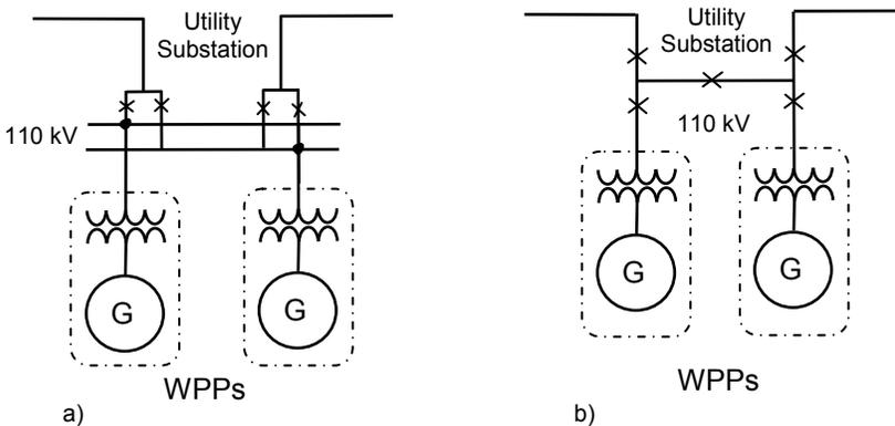
Figure 3.9 Methods for connecting Wind Power Plants to the National Power System:
