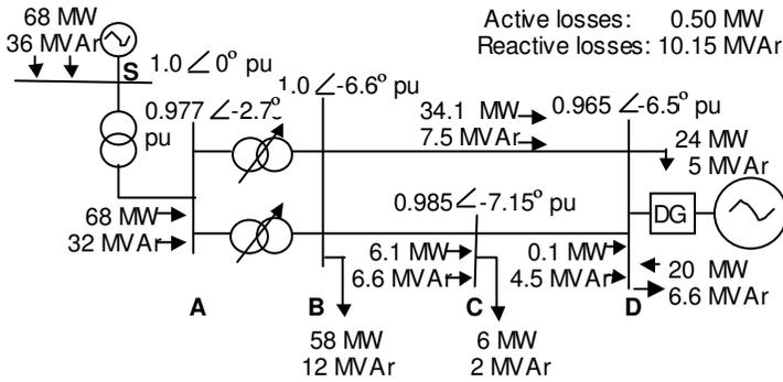
Figure 6.8 Power flow for maximum load and embedded generation at 0.95 power factor lagging (consumes reactive power)
