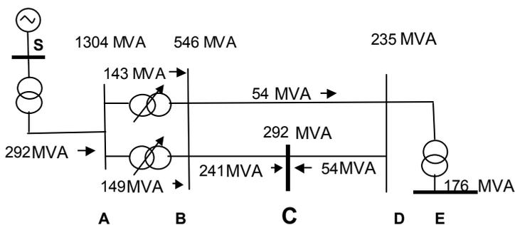
Figure 7.8 MVA fault levels for balanced three-phase faults at the various buses in the system. The arrows show the MVA flows for a fault at bus C. The system is assumed to be unloaded prior to the fault
