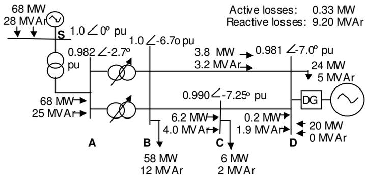
Figure 6.6 Power flow for maximum load and embedded generation at unity power factor
