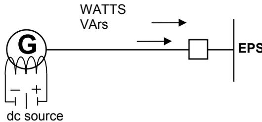
Figure 3.3 Synchronous Generator: dc field provides excitation, need to synchronize to utility system
