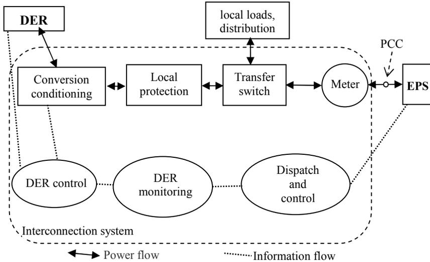
Figure 11.1 Interconnection system functional scheme - EPS - Electric Power System; DER - Distributed Energy Resource; PCC -Point of Common Coupling
