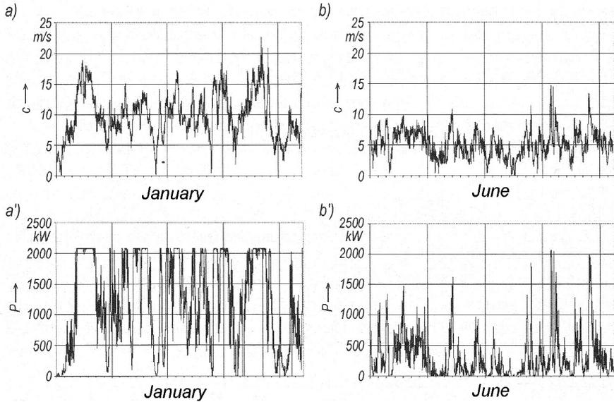
Figure 2.1 Wind speed diagram: vertical axis is wind speed  $c$ , 0-25  $\text{ms}^{-1}$  and power output  $P$ , 0-2.5 MW for WP in Kamięnsk PL
