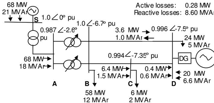
Figure 6.7 Power flow for maximum load and embedded generation at 0.95 power factor lagging (producing reactive power)
