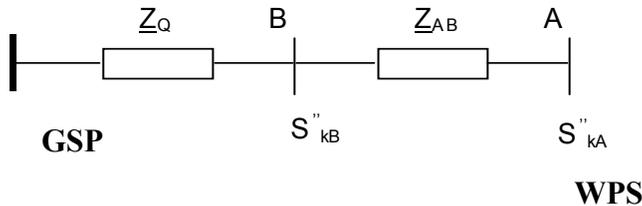
Figure 15.10. Model of a network equivalent for flicker
