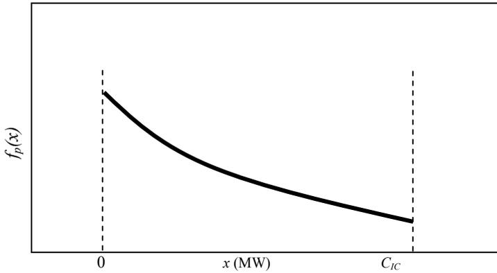
Figure 2.6 Probability density function for the available power production from several wind power units
