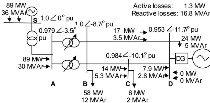
Figure 6.5 Power flow for maximum load and no dispersed generation
