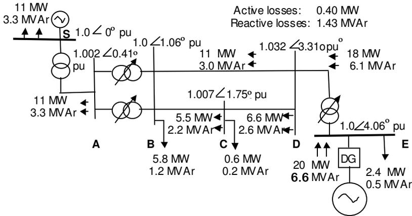
Figure 6.10 Power flow for minimum load and embedded generation at 0.95 power factor lagging on a voltage controlled bus
