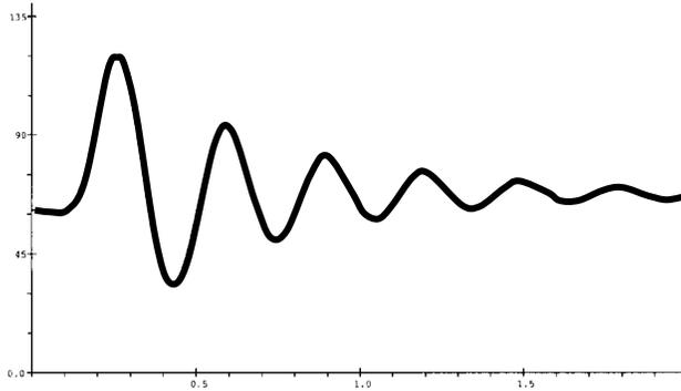
Figure 10.3 Oscillations in the rotor angle of the embedded generator at bus E following a fault at bus D when this generator produces 20 MW. The fault is applied at  $t = 100$  ms and cleared at  $t = 200$  ms
