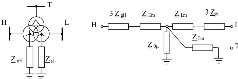
Figure 7.14. Three-winding transformer - the case of YNdyn
