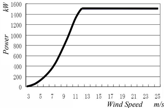
Figure 13.3 Power curve of the PMSG wind turbine
