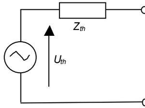
Figure 8.1 Thévenin equivalent circuit
