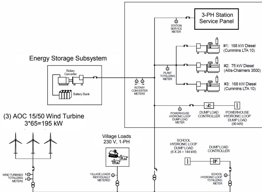
Figure 13.4 A sample of wind-diesel hybrid power system
