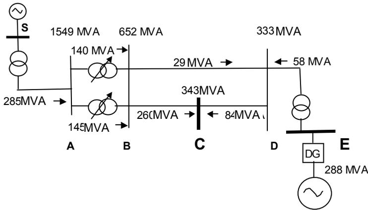
Figure 7.9 MVA fault levels for balanced three-phase faults at the various buses in the system, including the contribution of the embedded generator at bus E. The arrows show the MVA flows for a fault at bus C. The system is assumed to be unloaded prior to the fault
