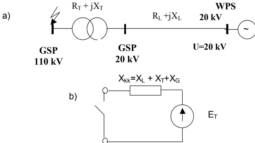
Figure 15.8 Schematic diagram (a) and equivalent circuits (b) used to designate for increase short circuit power at 110 kV substation, after grid connection of a wind turbine
