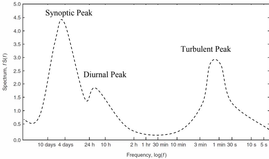
Figure 2.2 Power spectrum of wind speed variation
