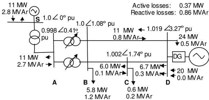
Figure 6.9 Power flow for minimum load and embedded generation at unity power factor
