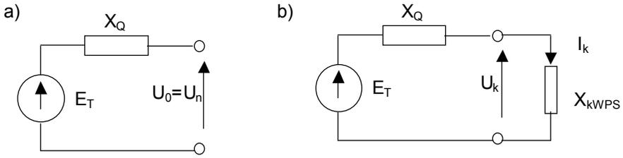
Figure 15.7 Two equivalent circuits for rapid voltage changes, a) before and b) after grid connection of a wind turbine
