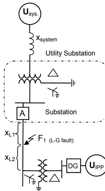
Figure 3.7 Single Line Diagram for Wye-Grounded/Delta Interconnection Transformer
