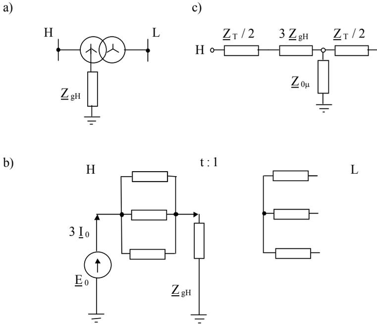
Figure 7.13 Case of YNy transformer windings, a) key diagram, b) measurement diagram, c) equivalent diagram.
