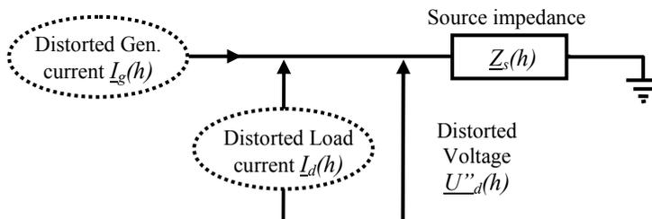
Figure 12.3 Effect of an embedded generator producing a distorted current on network power quality
