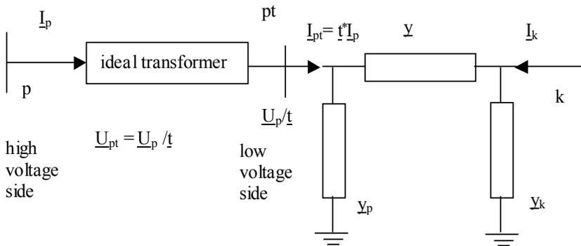
Figure 6.1. Scheme of transformer with on-load regulation
