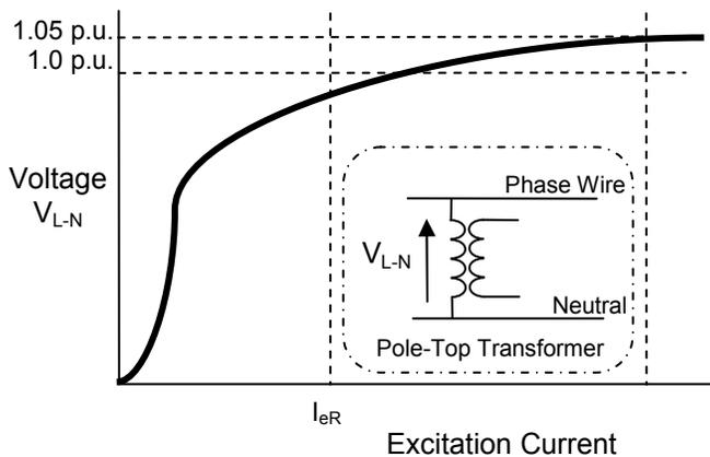
Figure 3.6 Saturation Curve of Pole-Top Transformer
