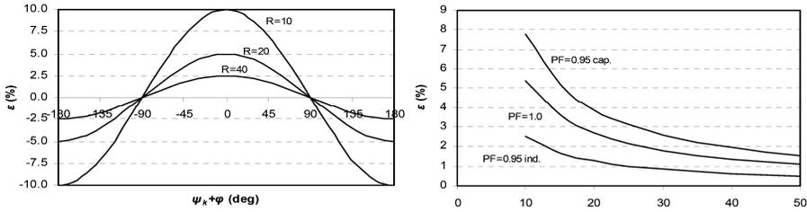
Figure 4.1 Voltage change  $\varepsilon$ (%) as a function of angle  $(\psi_k + \varphi)$ , for three values of the short circuit ratio  $R$  (left diagram) and  $\varepsilon$ (%) as a function of  $R$ , for three power factor values of the DG (right diagram) [21].
