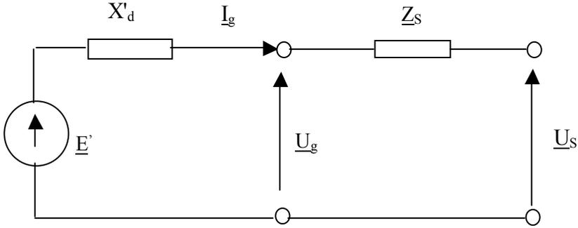
Figure 5.1. Equivalent scheme of generator in classical modeling.
