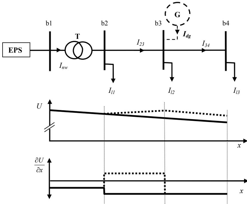
Figure 11.3 Voltage profile and gradient on a distribution feeder with and without contribution of generator G. Solid line:  $I_{dg} = 0$ , downstream power flow; dahsed line:  $I_{dg} > I_{l2} + I_{l3}$ , reverse power flow between  $b_2$  and  $b_3$ .
