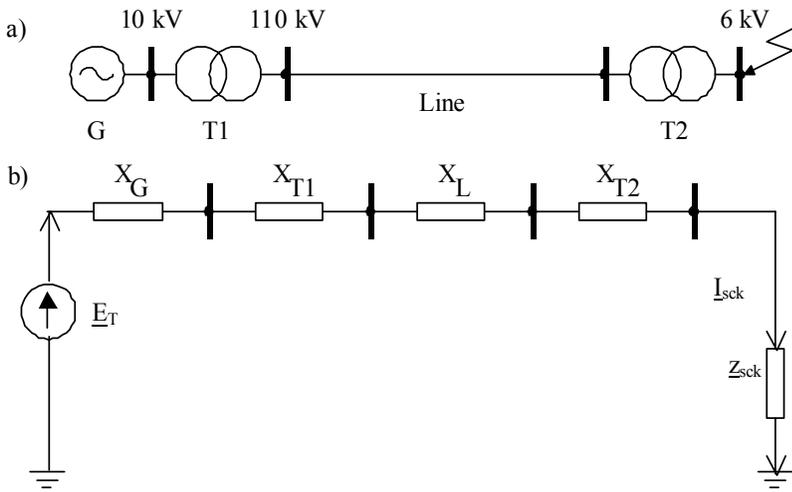
Figure 7.6. Single-phase representation of the 3-phase short-circuit in a system with a generator  $G$  connected through a transformer  $T1$ , a transmission line and transformer  $T2$  to a short circuit impedance.
