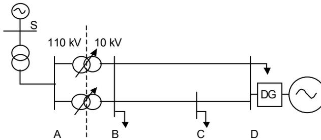
Figure 6.4 Portion of a distribution system with a dispersed generator. His network is connected to the transmission system at bus S and the dispersed generator is connected at bus D
