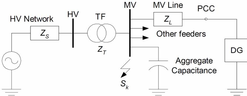
Figure 4.2 MV network equivalent for simplified harmonic emission evaluation
