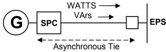
Figure 3.4 Asynchronous Generator: static power converter (SPC) converts generator frequency to system frequency, generator asynchronously connected to power system
