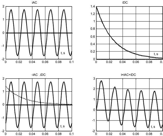
Figure 7.3. Time functions of a short-circuit current for the following circuit variables :
