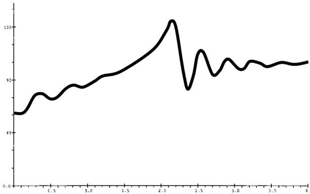
Figure 10.6 Oscillations in the rotor angle of the embedded generator at bus E following a fault at bus F when this generator produces 20 MW. The fault is applied at  $t = 0.1$  s and cleared at  $t = 2.1$  s
