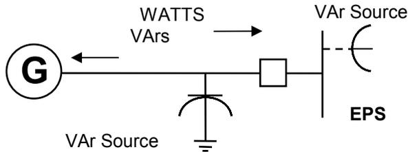
Figure 3.2 Induction Generator: excitation provided externally, start up like a motor (e.g. no synch. equipment needed), less costly than synchronous machines
