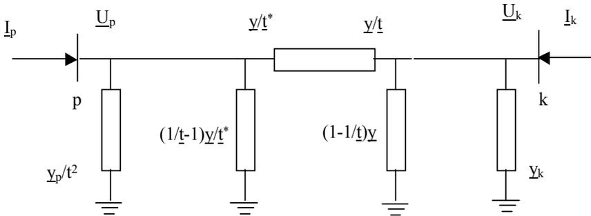
Figure 6.2 Equivalent circuit using fictitious shunt elements
