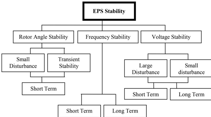
Figure 10.1 Classification of power system stability
