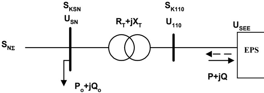
Rys.15.5. Scheme for the calculation of rapid voltage changes caused by the sudden shutdown of the wind farm.
