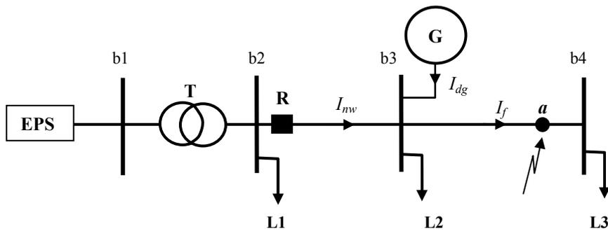
Figure 11.2 Short circuit at point **a**. Current from transmission network  $I_{nw}$ , current from embedded generator  $I_{dg}$ .
