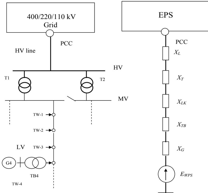
Figure 15.2. System circuit diagram and equivalent circuit for calculating the short circuit currents. Note PCC - Point of Common Coupling,  $X_L$  is the HV (110kV) line reactance,  $X_T$  110 kV/MV or HV/MV transformer reactance,  $X_{LK}$  - reactance of the internal network cable,  $X_{TB}$  is the total reactance seen from the primary side of the turbine booster transformers,  $X_G$  is the total reactance of all generators,  $E_{WPS}$  – *emf* of WPS.
