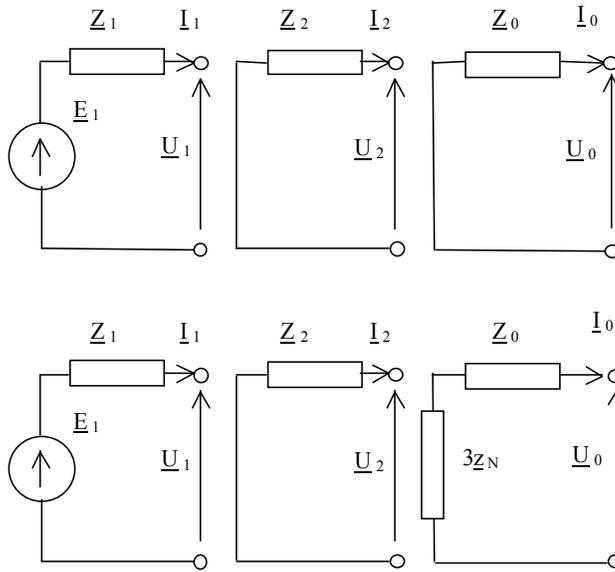
Figure 7.10 Scheme of generator sequence networks for a) the unloaded grounded generator
