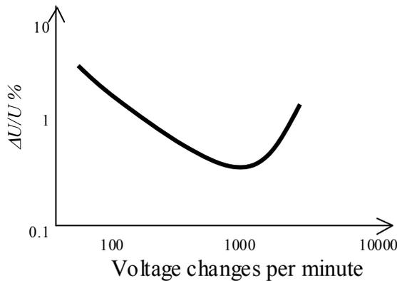
Figure 12.4 Influence of frequency and the perceptibility of sinusoidal voltage changes
