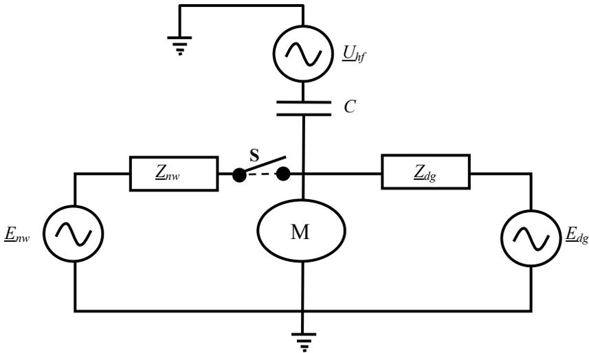
Figure 11.6: System impedance monitoring. The meter  $M$  will measure an increased HF signal when the utility network is disconnected
