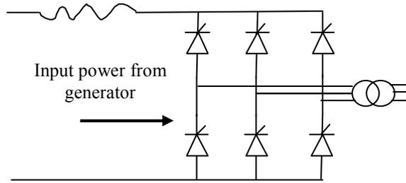
Figure 12.5 Line commutated converter
