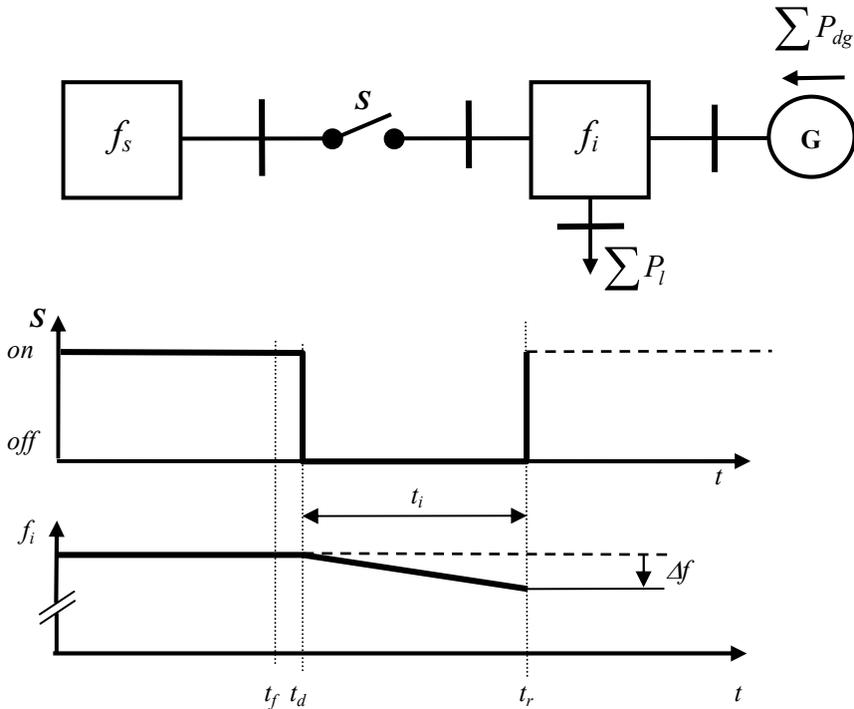
Figure 11.4 Auto reclosure procedure: fault occurs at  $t_f$ , disconnection of at  $t_d$ , reconnection at  $t_r$ , reclosure interval  $t_i$ ; state of utility switch  $S$ , utility synchronous frequency  $f_s$ , island frequency  $f_i$ , frequency drop  $\Delta f$ .
