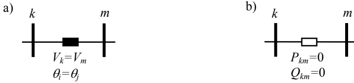
Fig. 11.5. Operational constraints for circuit breakers in the generalized state estimation: (a) closed circuit breaker, (b) open circuit breaker.
