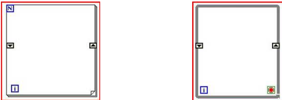
Fig. 10.9. Use of the shift registers with the “For Loop” and the “While Loop” structures
