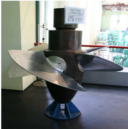
Fig 4.3. Propeller of the Kaplan turbine Source: www.wissen-mit-spass.de
