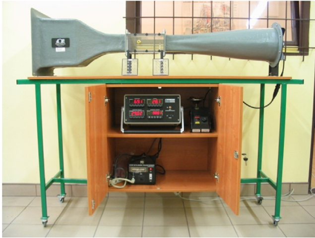
Fig. 2. Benchtop wind tunnel used for determining thermocouple time constant
