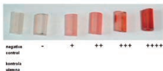
Fig. 1. The Richards's method – the level of colorless TTC reduction into the red-colored formazan on the catheter surface correlates with level of biofilm formation. The level of TTC reduction was estimated according to the following criteria: [-] lack of colour on catheter, [+] catheter surface is getting slightly pink; [++] redness of the whole surface; [+++] redness of the surface and the inside of the catheter; [++++] redness of the whole catheter, cloudiness and the red medium
