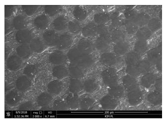
**Fig. 3.** Cross-section of a UHMWPE filament sealed with the composite material Magnification ×2,000.
