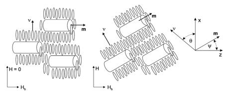
Fig. 2. Structure of ordered FN layer and its orientation change under influence of magnetic field ( $\nu$  – nematic liquid crystal director, **m** – unit vector of ferroparticle magnetization director,  $\theta$  – nematic molecule tilt angle,  $\psi$  – ferroparticle magnetic moment tilt angle).
