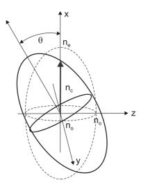
Fig. 3. Change of a spatial structure of the ferronemtic layer's refractive index ellipsoid ( $n_c$  – refractive index of FN layer for TM mode).
