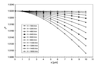
Fig. 4. Calculated refractive index profiles of FN layer for growing values of magnetic field intensity.
