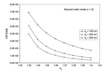
Fig. 7. Phase change of a second order TM mode in magnetic field of intensity H = 16000 A/m vs. refractive index of ordering layer  $n_p$  for different values of ordering layer thickness  $d_p$ .
