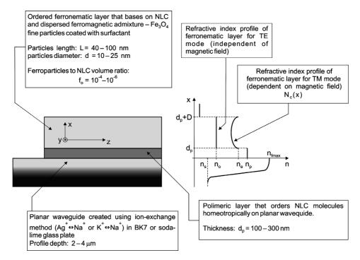
Fig. 1. Cross-section of a planar waveguide covered with a FN layer, the roles of individual layers and refractive index profiles for TE and TM modes ( $n_s$  – refractive index of substrate,  $n_p$  – refractive index of ordering layer,  $n_{f\max}$  – maximal value of refractive index in the waveguide layer,  $n_o$  – ordinary refractive index of FN layer,  $n_e$  – extraordinary refractive index of FN layer,  $d_p$  – thickness of ordering layer, D – thickness of FN layer).
