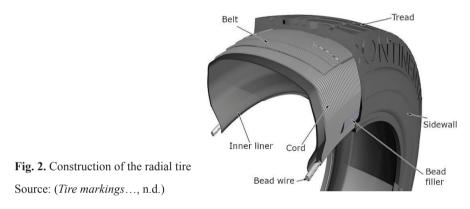
A number of components of both types of tires were described earlier, therefore only significant, different components of the radial tire are listed below (Jaworski, 1987; *Tire markings...*, n.d.):
