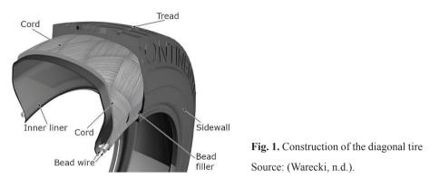
A diagonal tire is made with several layers of cord arranged alternately in two directions at an angle different than 90°. With this design, higher stiffness is obtained than in radial tires. The diagonal construction has advantages and disadvantages. The advantages are (Andrzejewski, 2010):
