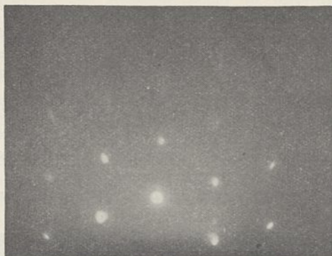
FIG. 2. Diffraction pattern due to etched single crystal of copper.
