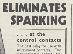
non-inductive control circuit eliminates the switching surge. For A.C. or D.C. circuits-currents up to 30 A-volts up to 600.
