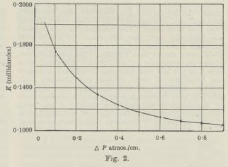
Fig. 2 shows the results in another form. The permeability, which is the tangent at each point of graph on Fig. 1, is plotted against the pressure differential. It is seen that instead of the constant value for permeability demanded by Darcy's law, a variable permeability is obtained, falling to an assymptotic value at higher rates of flow. The assymptotic value is what is usually obtained in permeability measurements using fairly high rates but necessarily limited to the viscous regime.
