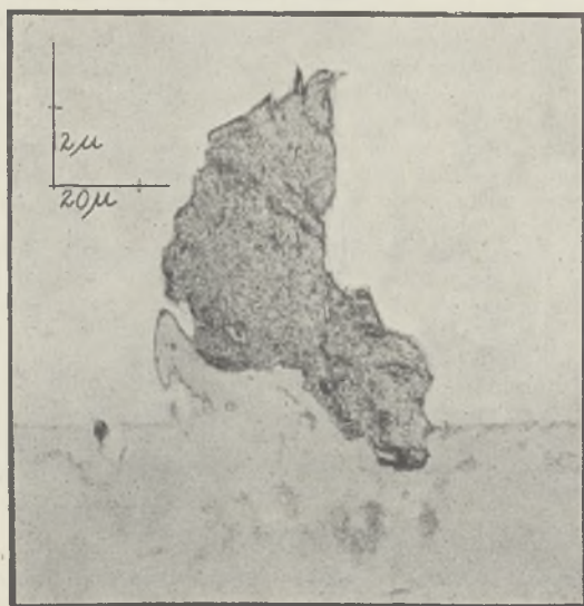
Fig. 1. TAPER SECTION SHOWING COPPER FRAGMENT (DARK) WELDED ON TO STEEL SURFACE; NOTE PLUCKING UP OF STEEL. VERTICAL, \times 5000 ; HORIZONTAL, \times 500 .
