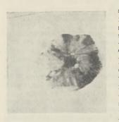
Associated with the stronger reflexions there is frequently found a streak extending sometimes on both sides of the central position. This is due to the 'angular spread' of the polycrystalline material at the reflecting spot. This method is therefore a for convenient one studying variations of texture of the material, which include relatively
