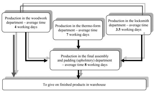
Figure 2. Production process with manufacturing times in each department
