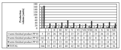
Figure 5. Equalized plan of workload for production positions for semi-finished products PP 01, PP 02, PP 03
