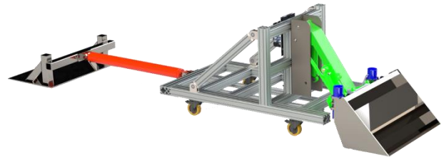
Figure 4. CAD Model Wheel Loader Test Rig [GUS22]
