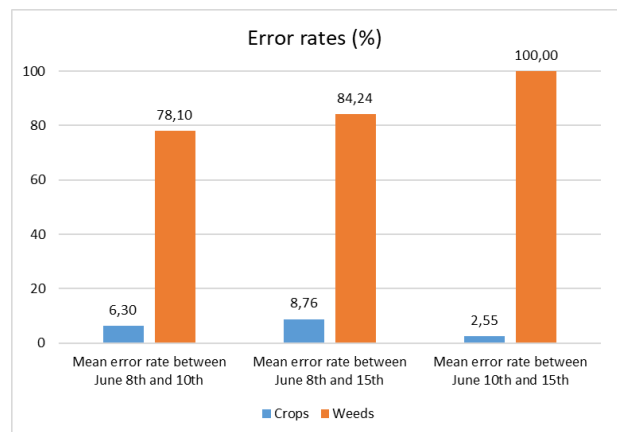
Figure 2. Intra-row weeding results on the bean/rye-grass plot for the only team who participated
