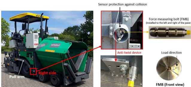
Figure 3. Illustration of the force measuring bolt installed at the traction point of the pull arm for recording the traction force
