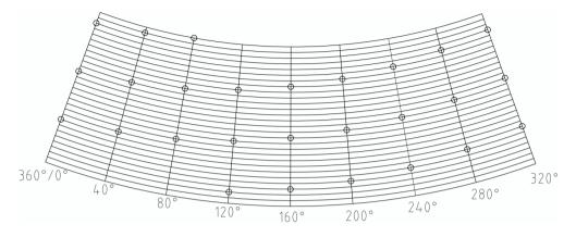
Fig. 4. Lateral expansion of pick arrangement
