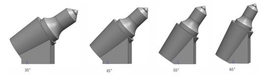
Fig. 1. Cutting angle of picks
