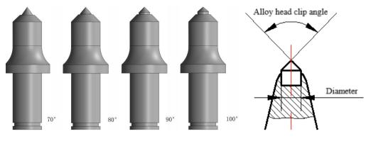
Fig. 7. Alloy head clip angle
