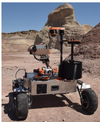
Fig. 1. Scorpio 7 mobile research platform with installed Raman spectrometer (spectrometer is located under black, round cover)
