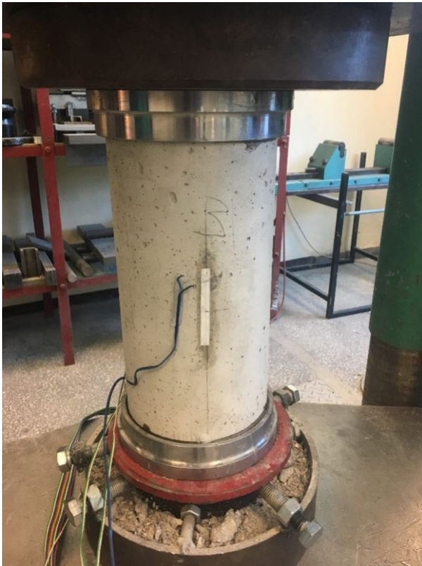
Figure 5: Concrete specimen placed in strength-testing machine.
