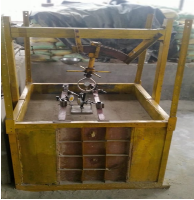
Figure 5: Experimental set up for 5° angle of inclination.
