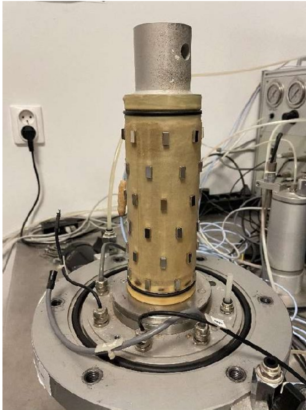
Figure 6: The sand specimen covered with a latex membrane and magnets attached to the surface. The main RC tests were carried out with the input parameters presented in Table 2 .
