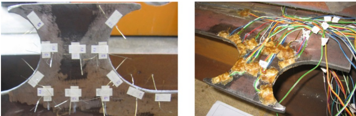
Figure 12: Strain gauges on NPOT specimens with CL shapes for purposes of [7].
