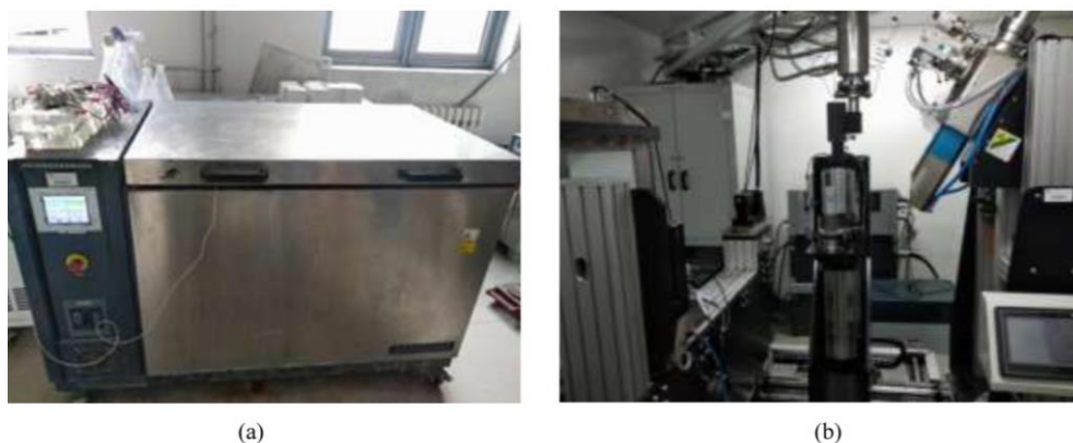
Fig. 2. Main equipment used: (a) Freeze-thaw machine, (b) Micro Focus X-ray CT Scanning Equipment
