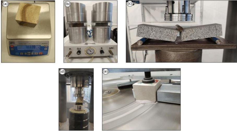
Fig. 3. Some of the laboratory studies: a) determination of the oven-dried weight for a cubical rock sample, b) Determination of w_a , c) FS test, d) UCS test, e) BAV test
