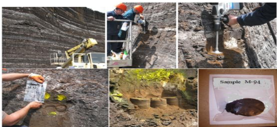
Fig. 4. In-situ sampling procedure on coal cascades
