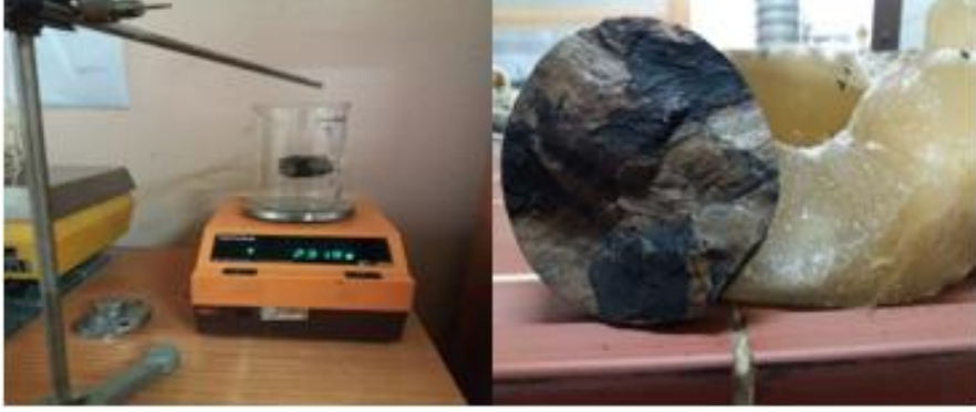
Fig. 8. Determination of volumetric weight with paraffin
