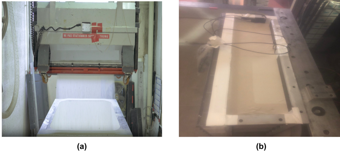
Figure 1. Sand preparation process: (a) sand raining technique and (b) prepared strongbox.
