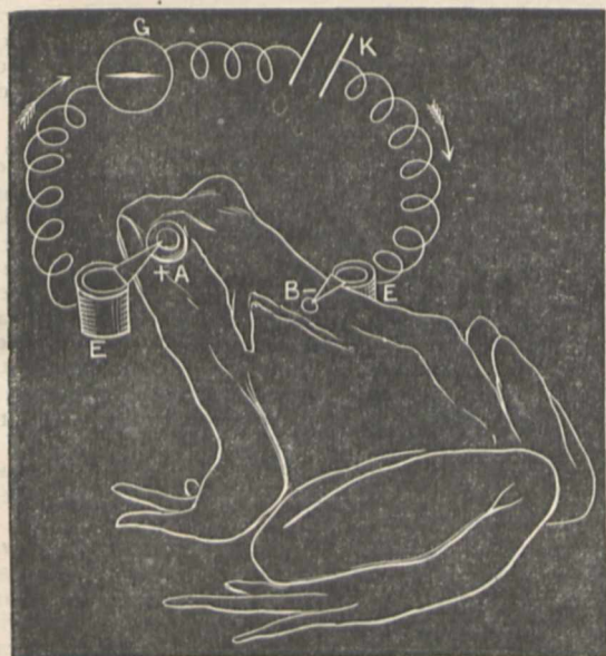
Diagram showing arrangement of apparatus in the experiment on eye of frog. A, Eye showing the electrode, e , in contact with it. B, Skin removed, and subcutaneous tissue in contact with other electrode, k . K, Key. E, Galvanometer. Arrows indicate direction of current. Cornea, positive. Back, negative.
