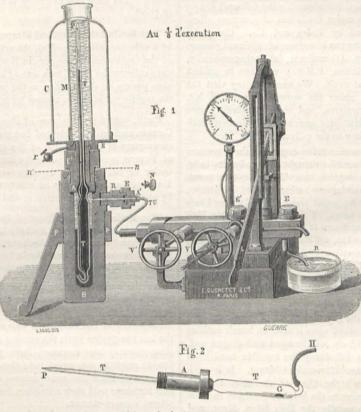
upon leather. The safety-bell-jar C is movable; it is intended to stop the pieces of glass should the tube T be broken. The stop-cock r lets the water flow from the envelope M. The lateral screw with the tube A' is refixed, to which is soldered the small metallic tube T V, by which pressure is introduced.
