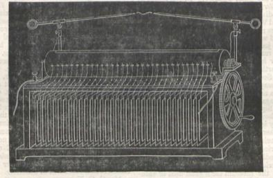
The tension of a secondary battery of 800 couples is not necessary to produce marked effects with this apparatus. By putting in action only 200 couples, we have sparks of eight millimetres, and we may, without doubt, by diminishing still more the thickness of the insulating plates and multiplying the number of condensers, obtain effects with a source of electricity of less tension.
