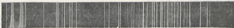
FIG. 4.—Part of the blue region in the spectrum of a mixture of incandescent aluminium, calcium, and iron vapours, showing how the images of the slit produce the appearance of bright lines.
