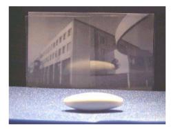
Fig. 7. Glaze of a white object placed in front of a AS-AG coated plastic (left) and an uncoated one (right). The picture of the building placed 2 cm behind the substrates is clearly visible in both configurations
