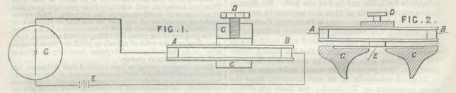
be very sensitive on a reflecting galvanometer I thought that probably the tube would be a means of transmitting articulate speech. I find this to be the case. Fig. 2, AB, elastic tube similar to the one used in the former instrument; CC, mouth-
