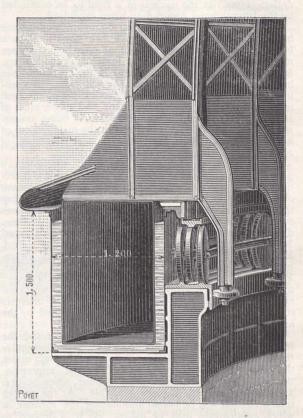
The annular caisson, which receives the floater and the liquid, has a rectangular transverse section ; its height is 1'50 m., and breadth 1 20 m. The latter dimension thus exceeds the breadth of the floater by 0'25 m., which gives a lateral play of 0'125 m. in the inside and 0'125 m. at outside between the floater and the caisson. Finally, the caisson rests on thirty-six strong cast-iron supports, distributed at equal distances over the upper part of the mason-work of the tower.
