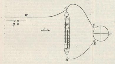
plate is connected with a platinum wire which may either be soldered to the plate or passed through a small hole in the plate and pinched tightly to it; these wires pass through the ends of the glass tube and are sealed into it. The poles of the cell are A, B, and these are connected with the poles of a quadrant electrometer (Clifton's form of Thomson's).
