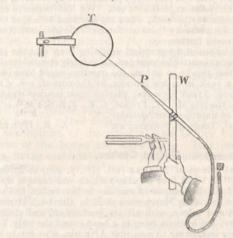
A tuning fork held in one hand is made to touch the lath held in the other while vibrating, and the whole moved nearer to or further from the tambourine.
