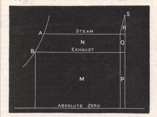
The vertical ordinates here are absolute temperatures, and the area is heat or energy. Without superheating, Carnot's law gives, between temperatures A and B-
