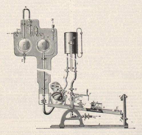
Thus, as already described, the water current is now cut off, the water present in M flows out through  $K_2$ , and the mercury goes back from the pump Q into the ball H.
