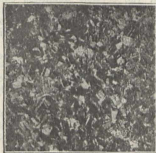
FIG. 2.—Alloy containing copper 80 per cent., zinc 20 per cent., annealed at 700^{\circ} .
