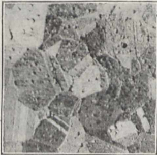
FIG. 4.—Commercial brass, containing traces of lead and tin, "burnt" by being annealed at 820^{\circ} .
