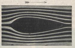
F13. 9.-Section of screw shaft s rut (broad colour bands in thin sheet).
