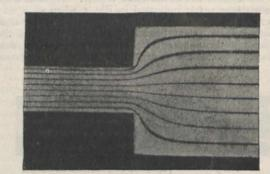
FIG. 14.-Sudden enlargement (thin sheet).
