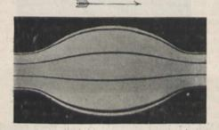
FIG. 12.-Colour bands in gradually enlarging and contracting channel (thin sheet).
