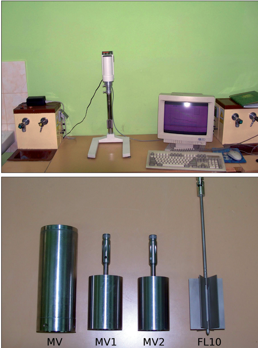
Fig. 2.1. Viscometer Haake VT550 and basic measurement systems
