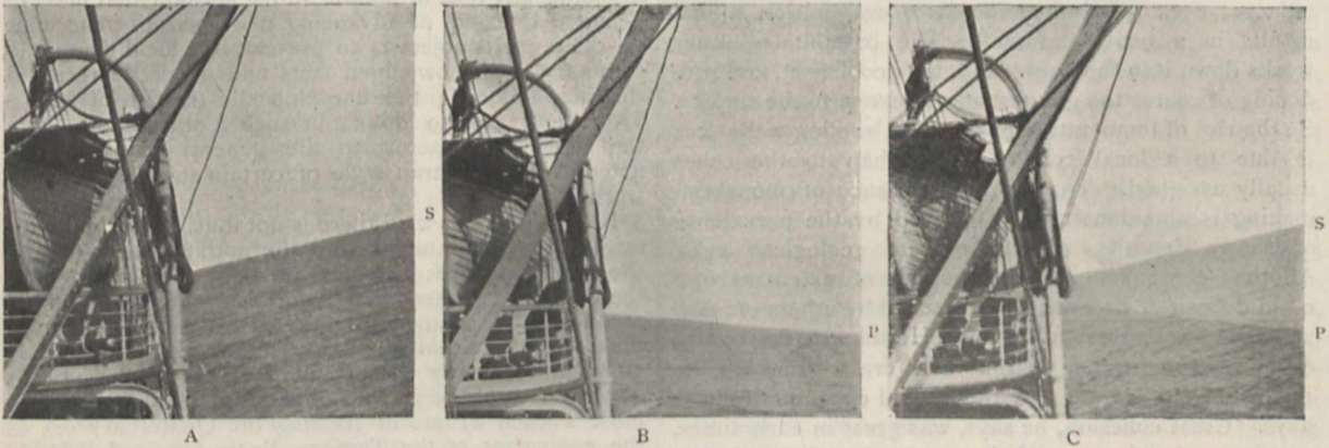
Union Steamship Co.'s Mokoia . Rolling angle found by photography. A is a picture taken at the instant of the end of rolling to the right, s; B is a picture taken at the instant of the end of rolling to the left, P; C is a composite picture made by superposing the two films, A and B. The pictures of the ship are made to coincide, thus the angle between the two horizons in A and B is found. Lat. 34° 27' S. Long. 157° 43' E. To Sydney 325 miles.
