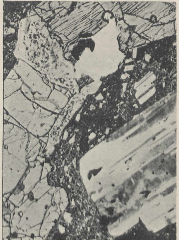
FIG. 1.—Hyalopilitic Hypersthene-Andesite; thin slice photographed in polarised light, magnification about 20 diameters.
