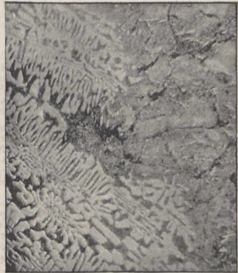
FIG. 8.—Pure Iron-Iron Carbide Eutectic, the cooling of which was arrested before the complete decomposition of the Carbides into Austenite and Graphite. White=carbide of iron. Black lines=graphite. Half-tone=pearlite.
