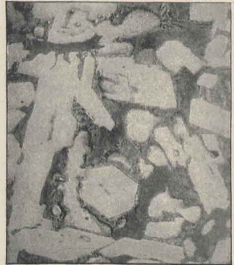
FIG. 6.—Glazed Cleveland Iron after melting with a little Sulphide of Iron. White crystals=primary carbo-silicide of iron. Dark=the second cementite. Complex structure=iron-carbon-phosphorus eutectic.
