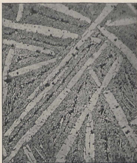
FIG. 3.—Iron-Carbon-Sulphur Alloy (4.37 per cent. Carbon). White thick bands=massive carbide of iron. Complex structure=iron-iron-carbide-sulphide-pearlite eutectic.
